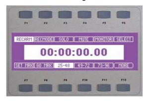
The first fixed LCD page determines the function of the track select keys and sets and locates Markers.
