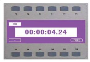
This page shows up to 5 machines on **F1** to **F5** (**F1**, the Internal Machine, is always present). Pressing **F1** to **F5** selects the corresponding machine. **F7** to **F11** labels show the current chase status of the machine above. Pressing F7 to F11 controls the CHASE state of the corresponding machine. Pressing SHIFT plus
