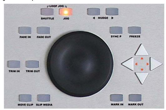
SHUTTLE = Jog Wheel Mode - Shuttle + SHIFT = Jog Wheel Mode - Jump
