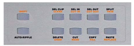
**SHIFT Shift (Fixed Assignment)** = **AUTO-RIPPLE** = **Auto-Ripple** Select Clip(s) under Cursor **SEL CLIP Undo Selection SHIFT CLEAR** = **Set Selection Start to Cursor SEL IN** = **SHIFT CUT IN Trim In to Cursor SEL OUT Set Selection End to Cursor** = **SHIFT CUT OUT Trim Out to Cursor** = Split Clip(s) at Cursor **SPLIT SHIFT TRIM** Trim **DELETE Delete SHIFT UNDO** Undo = **CUT** Cut = **SHIFT REDO** Redo **COPY** Copy = **SHIFT FILL Fill Selection**
