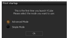
The Simple Mode has been designed to avoid inexperienced users destroying a correctly configured setup. But several settings are not accessible.
