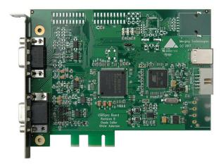
The Sync Board hardware option enables RS-422, LTC, MIDI (MTC) input and optional Bi-Phase input to control or to be controlled by VCube.
